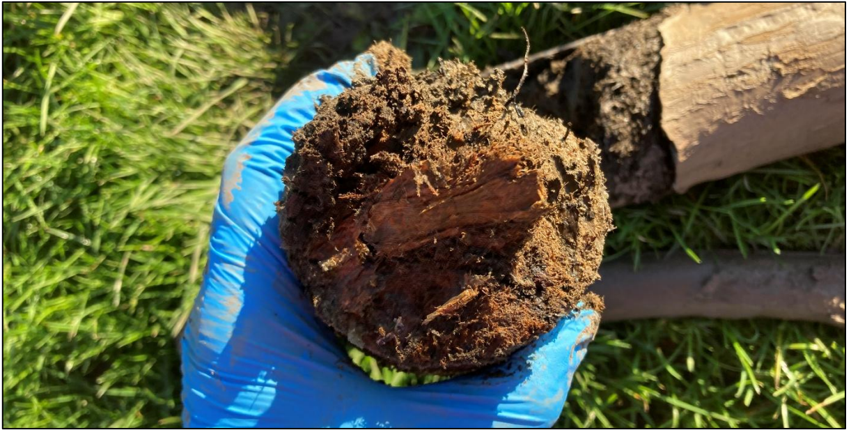
Figure 5-B: Made Ground extracted from WLS01, encountered between depths of 1.90 m to 3.00 m bgl
