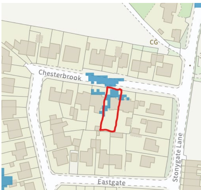
Figure 2 Extract from Surface Water flood depth map showing that flooding will be less than 20cm 07/05/2025
