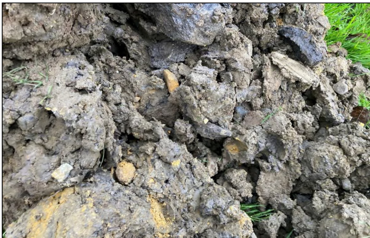
Figure 5-B: Devensian Till extracted from HP04
