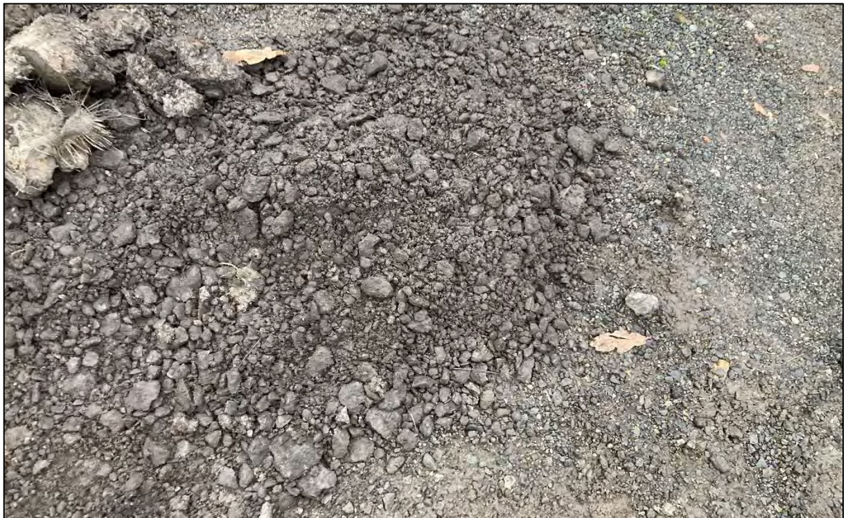
Figure 5-B: Gravel surfacing (Made Ground) encountered in HP07
