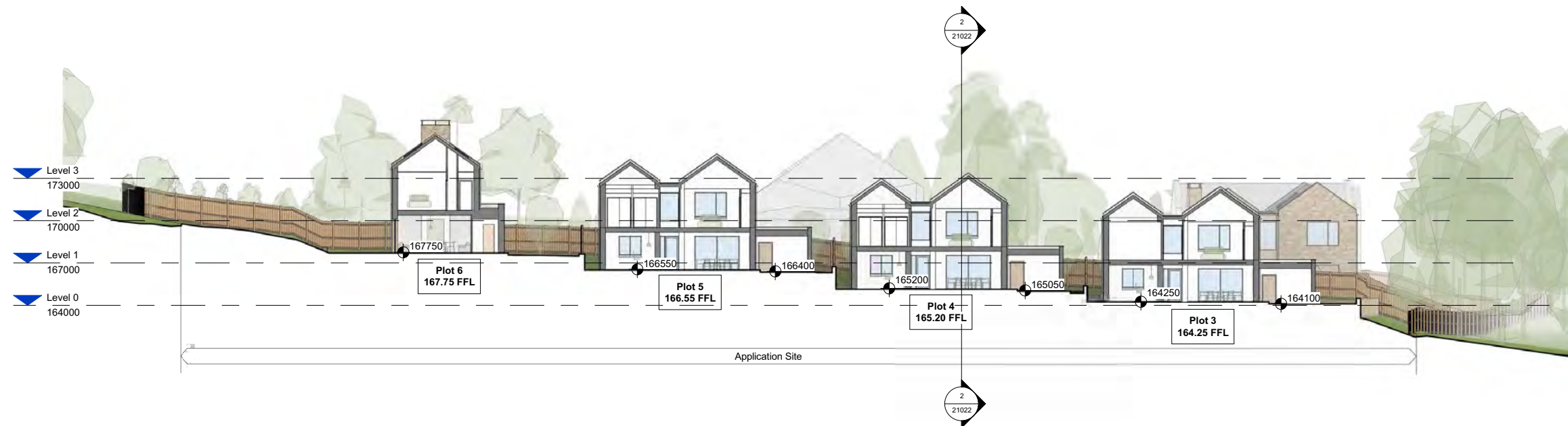
3 | Proposed Long Section along Site Slope 1 : 200
