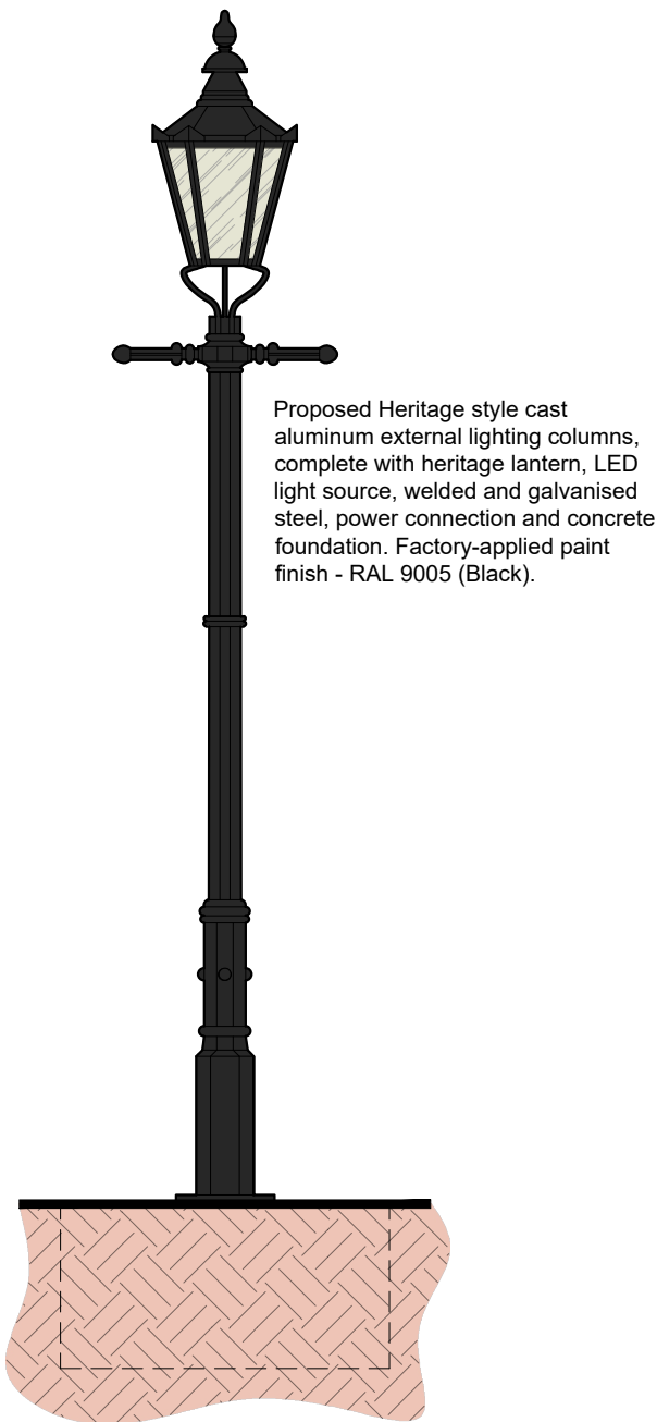
PROPOSED EXTERNAL LIGHTING COLUMN SCALE 1:20
