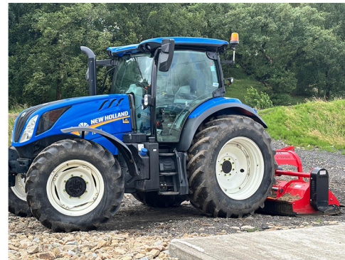
New Holland 6180 tractor (with flail mower attachment) 7.9 x 3.3m
