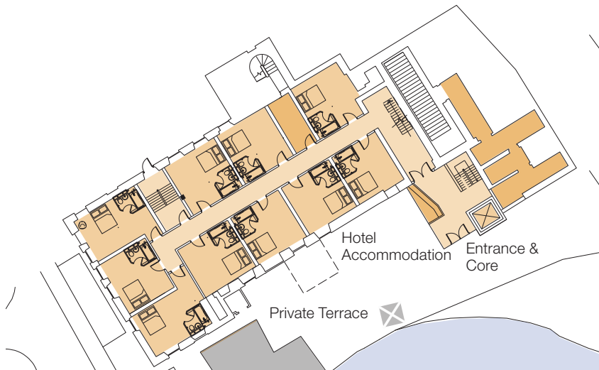
An early ground floor plan showing hotel accommodation and external circulation core at the front of the building.
