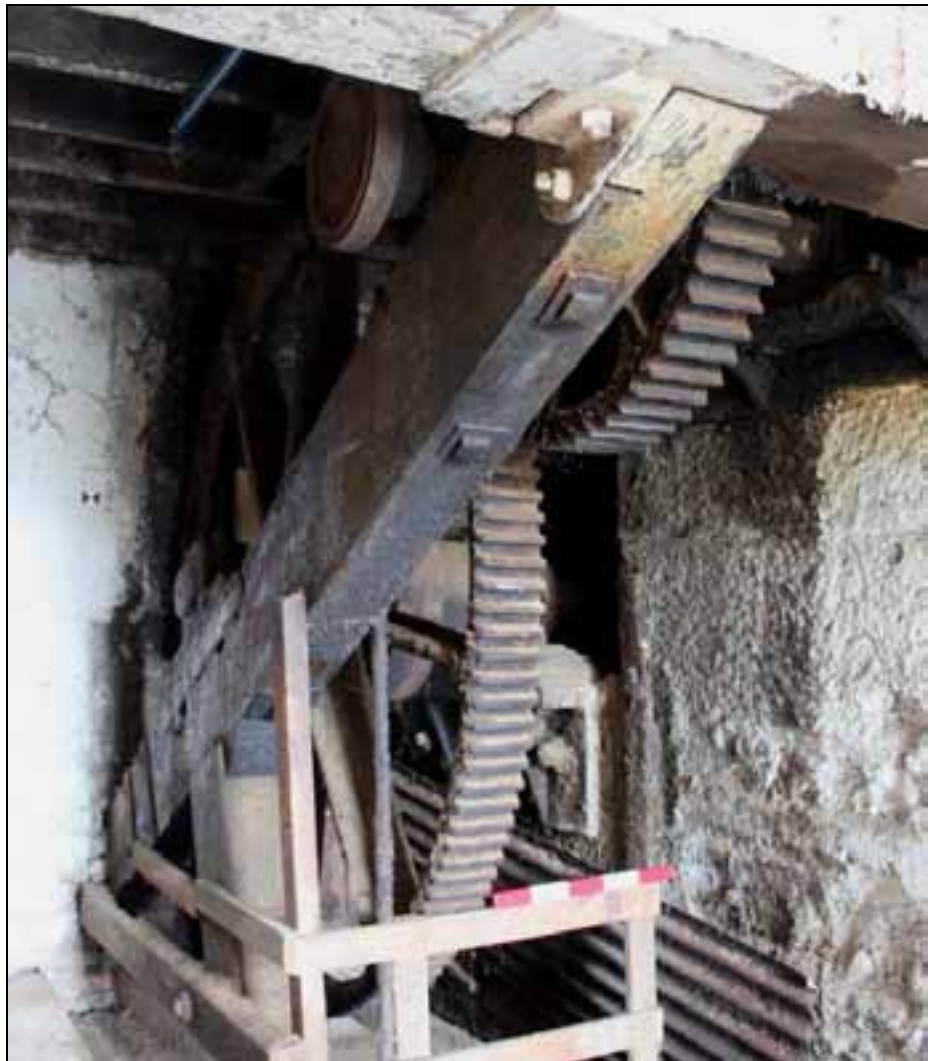
Plate 67: Gearing driven by pinion wheel, with clutch-plate on drive shaft
