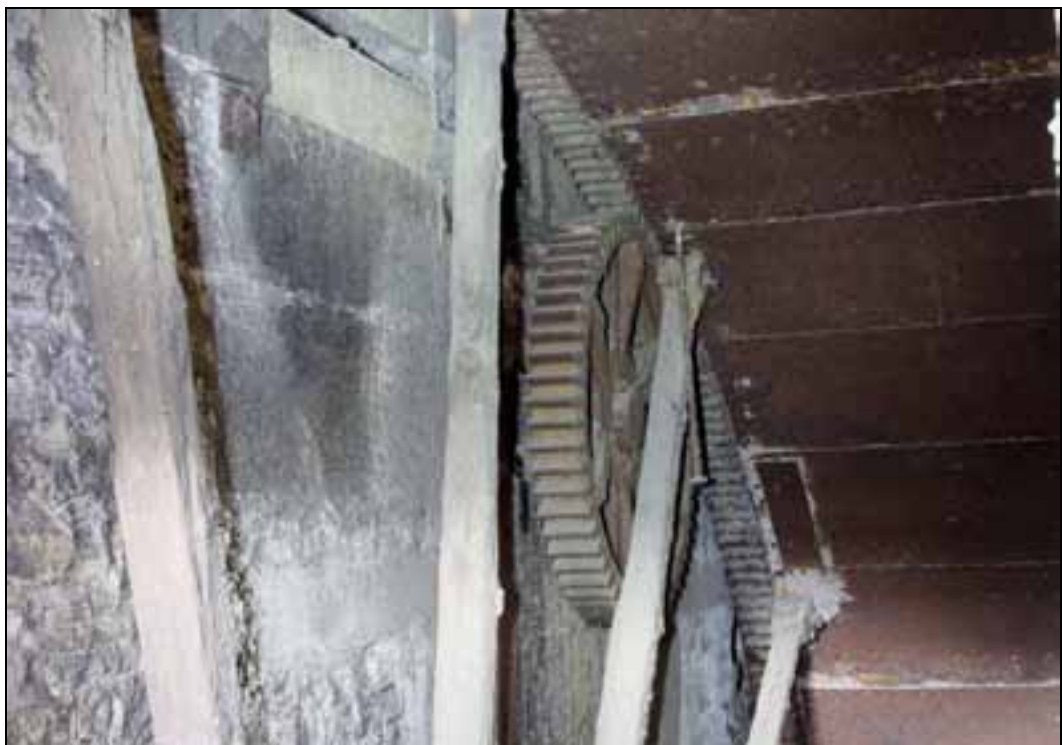
Plate 64: Pinion wheel on rim gear of waterwheel
