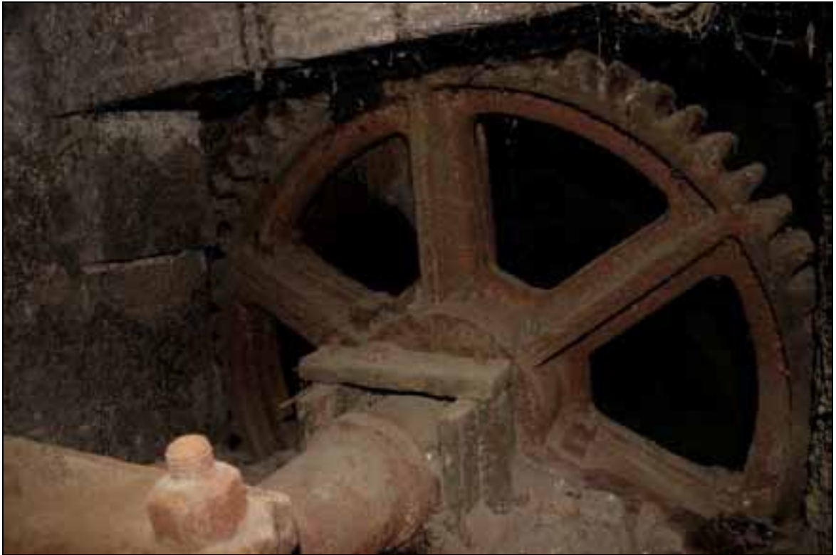
Plate 65: Axle and bearing of pinion wheel
