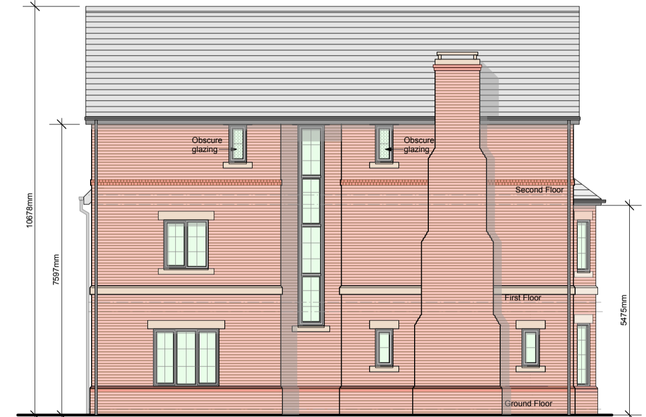
Side Elevation - North East
