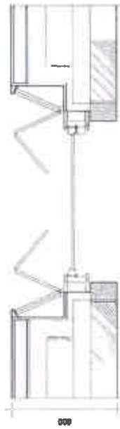
Plan of Sash Window 1:20
