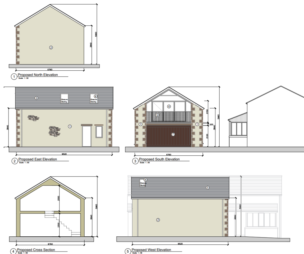
Figure 4.2: Drawing ref no. P.05-XX-002 – elevation details of proposed development
