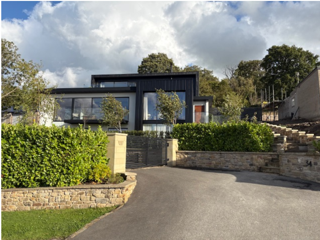
No 34 – Render, Zinc cladding, aluminium windows, corten steel door
