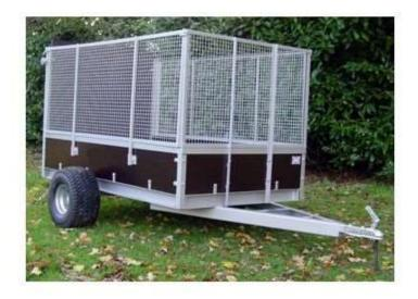
This trailer is a general purpose "off road" trailer for use behind quad bikes, ATV's etc.
