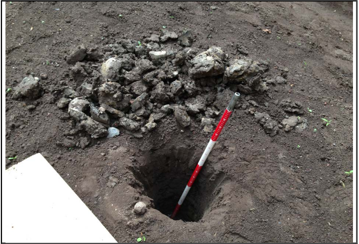
Plate 3 – Plot 20 Cover System Depth & Arisings
