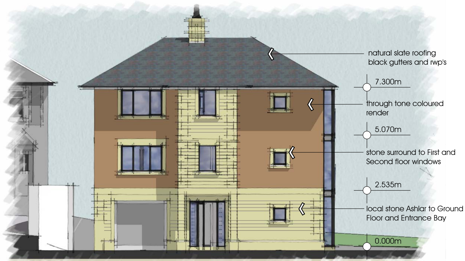
South West Elevation
